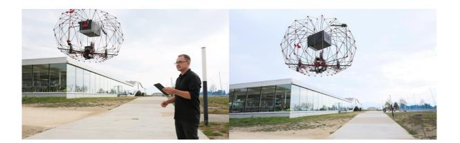
By adding such a cage to a multicopter, the team ensures safety for those who come into contact with the drone. The drone can be caught while it's flying, meaning that it can deliver to people caught in places where landing is hard or even impossible, such as a collapsed building during search and rescue missions, where first aid, medication, water or food may need to be delivered quickly.
