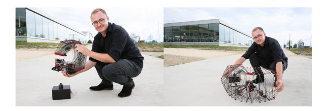
A foldable protective cage sits around a multicopter and around the package to be carried, shielding spinning propellers and ensuring safety of all people around it. When the folding cage is opened in order to either load or unload the drone, a safety mechanism ensures that the engine is cut off, meaning that safety is ensured, even with completely untrained users.
