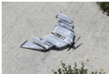
Rotating wingerons allow the robot to walk (Photo: © LIS/EPFL and Alain Herzog 2014).
