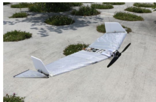
The DALER extends its wings to fly (Photo: © LIS/EPFL and Alain Herzog 2014).
