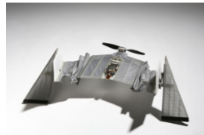
The DALER uses wings inspired by bats (Photo: © LIS/EPFL and Alain Herzog 2014).
