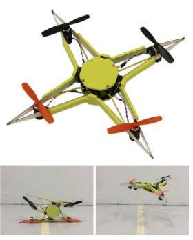
back after the collision, allowing the frame to realign and thus ensuring that the drone is once again ready to fly.
