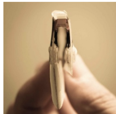
The actuator can be completely folded in half without damage
